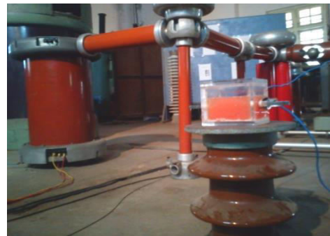
Fig.15 : Static treatment Chamber
