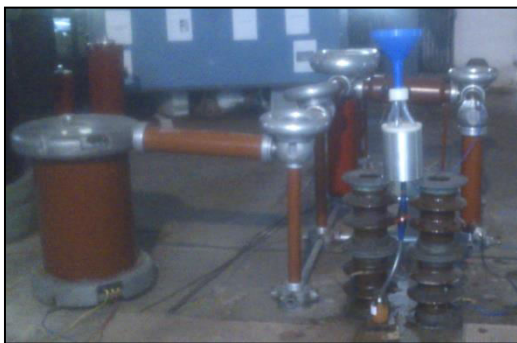
Fig.16: Co-axial Continuous flow treatment chamber.
